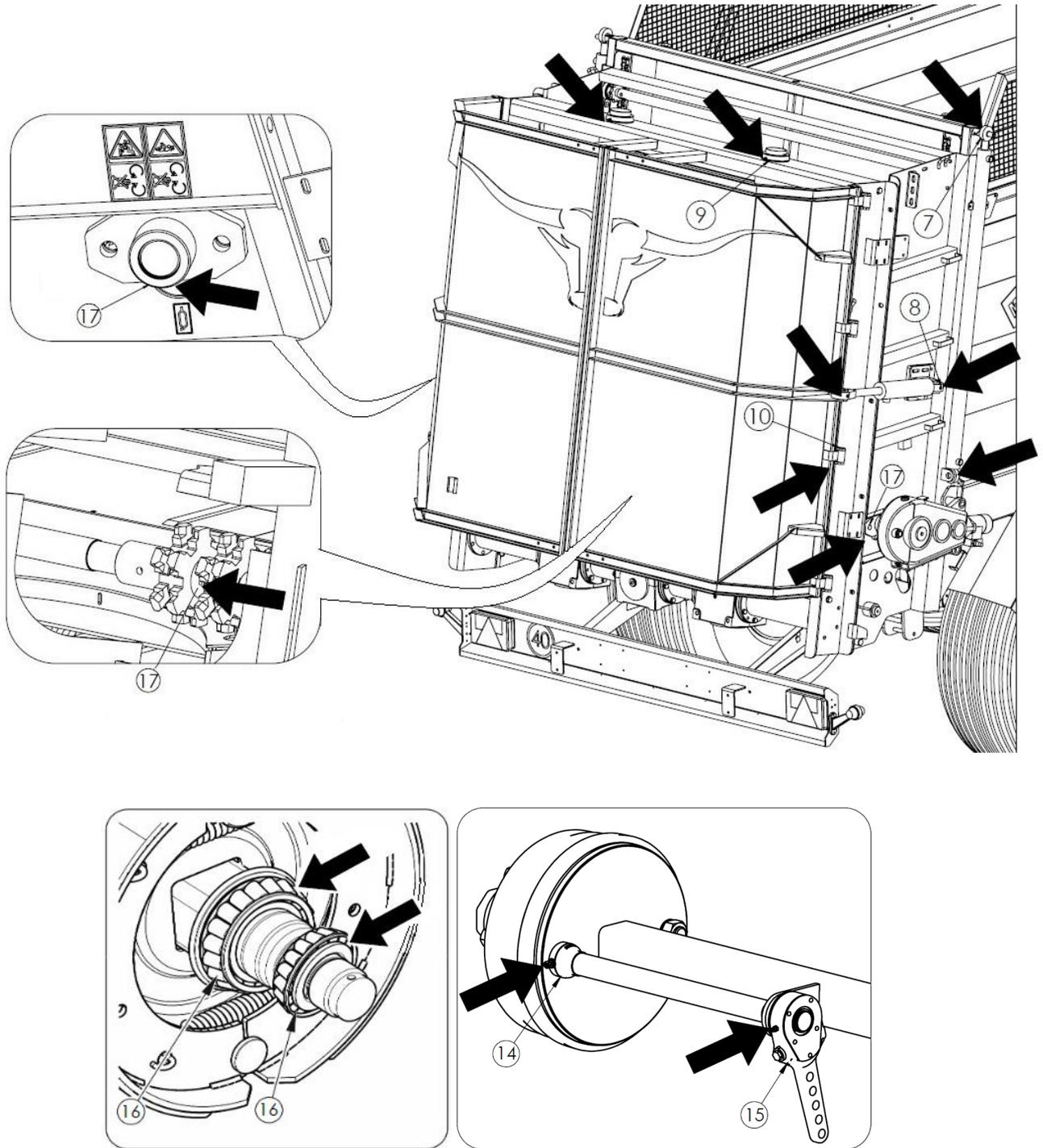
**Figure 35.** Spreader lubrication points
