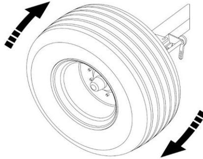
**Figure 41.** Checking wheel bearing play
