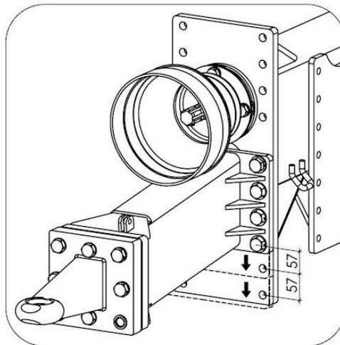
**Figure 19.** Adjusting the hitch height
