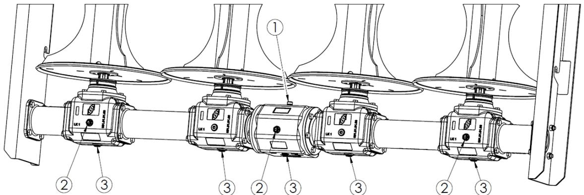
**Figure 32.** Oil level control points in the 4-auger adapter gearbox
