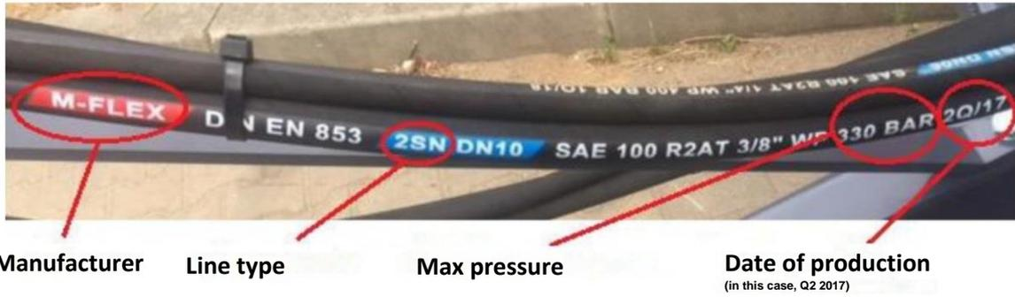
**Figure 21.** Marking of the hydraulic lines
