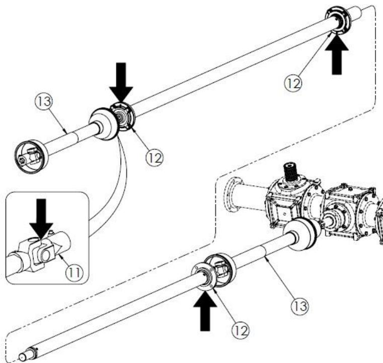
**Figure 34.** Spreader lubrication points
