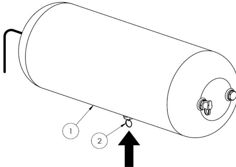
**Figure 40.** Draining the air tank:
