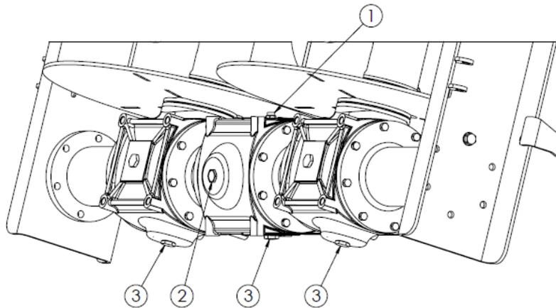
**Figure 31.** Oil level control points in the 2-auger vertical and 2-auger horizontal disc beater unit gearboxes
