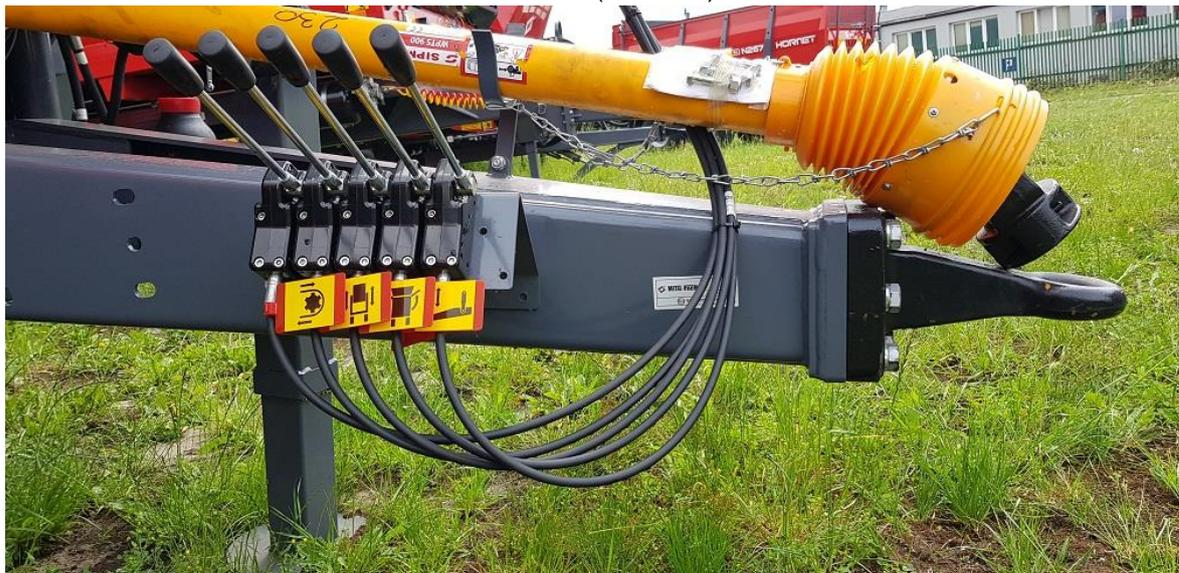
**Figure 23.** Pictograms for the control levers of the distributor (distributor control is optional)
