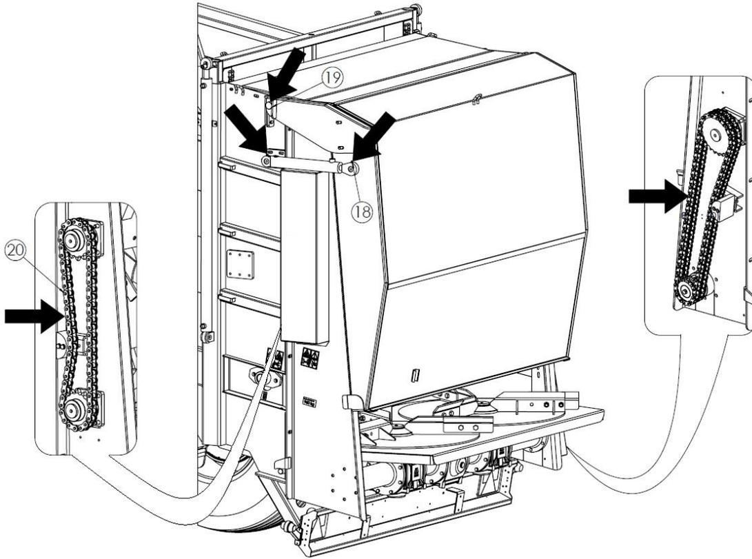
**Figure 36.** Spreader lubrication points (2-auger horizontal disc beater unit)
