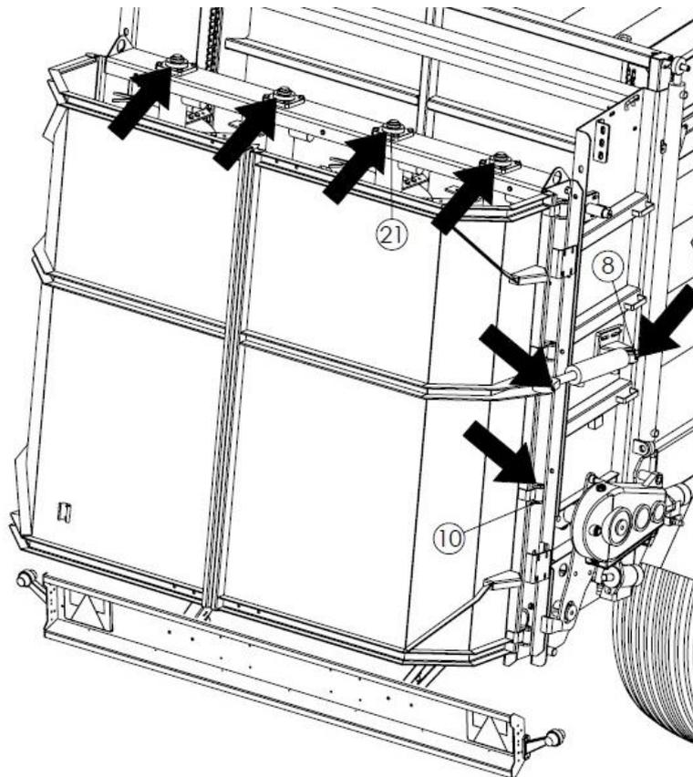
**Figure 37.** Spreader lubrication points (4-auger vertical beater unit)
