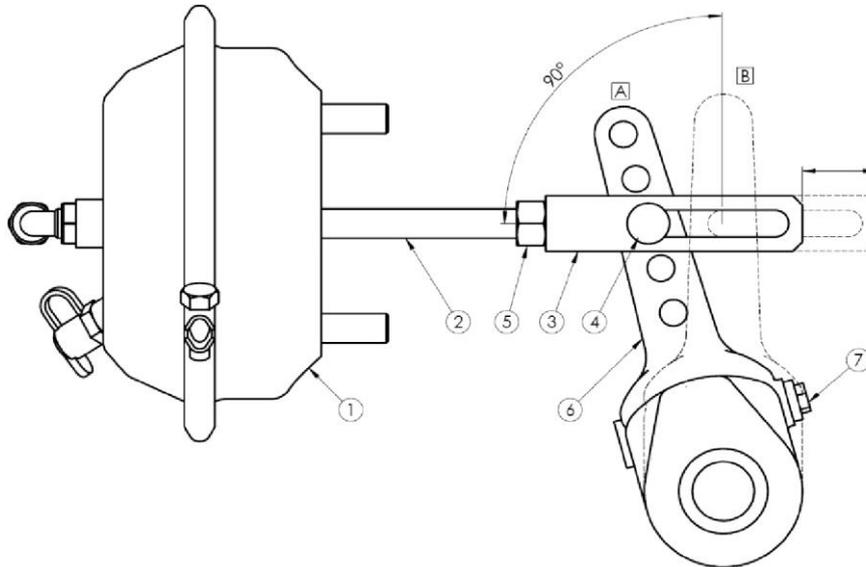
**Figure 43.** Adjustment of the parking brake
