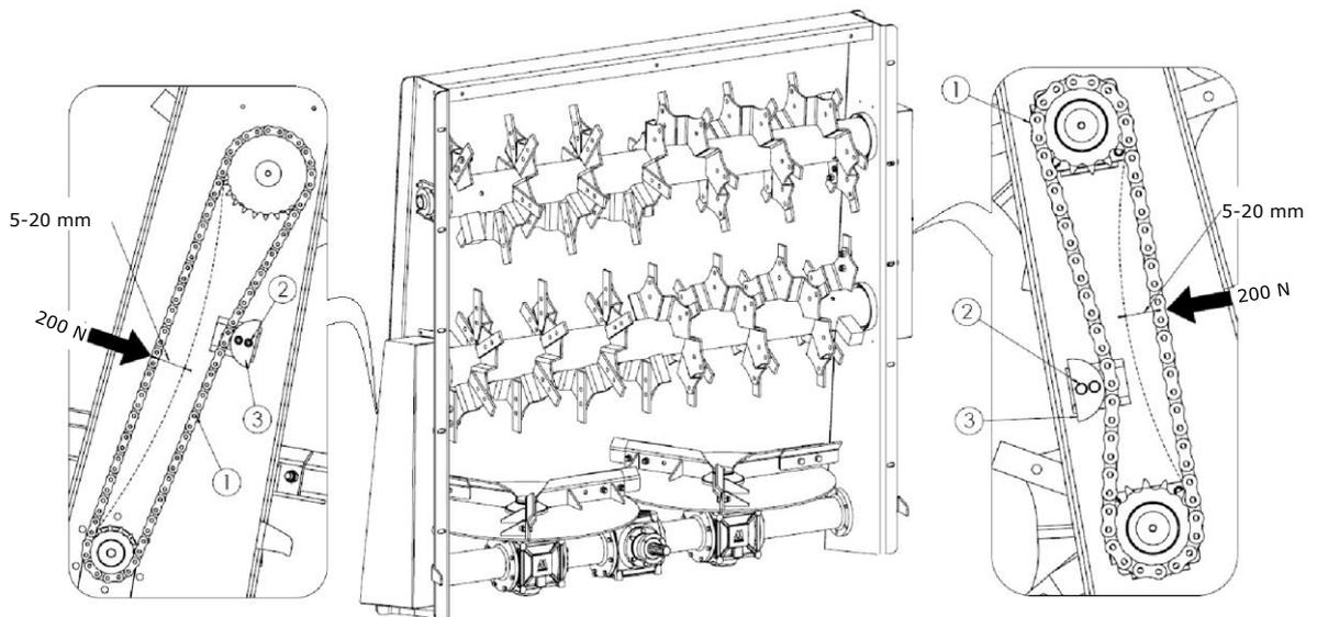
**Figure 29.** Tensioning the beater unit chains
