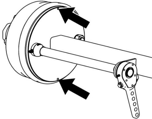
**Figure 42.** Inspections of the brake linings for wear
