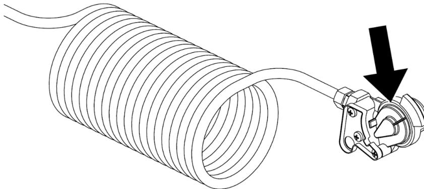
**Figure 38.** Haldex brake system air filters
