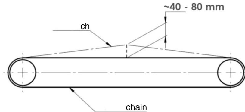
**Figure 28.** Checking the tensioning of the spreader chains
