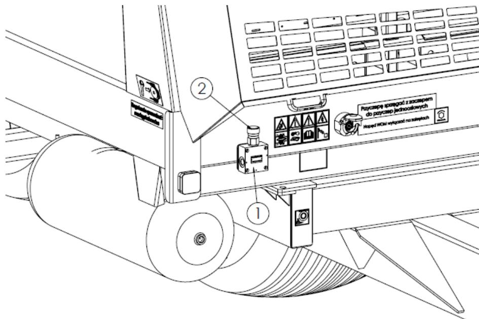
**Figure 24.** Adjusting the travel speed of the floor conveyor:
