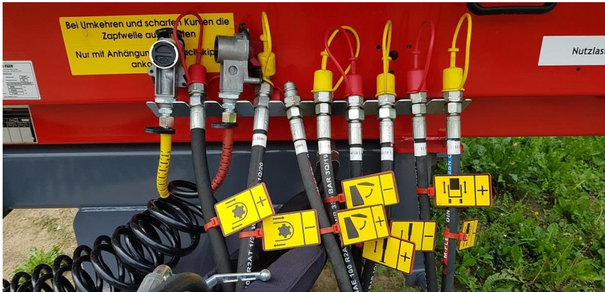
**Figure 22.** Pictograms on the hydraulic connectors for easier connection to the tractor (standard)
