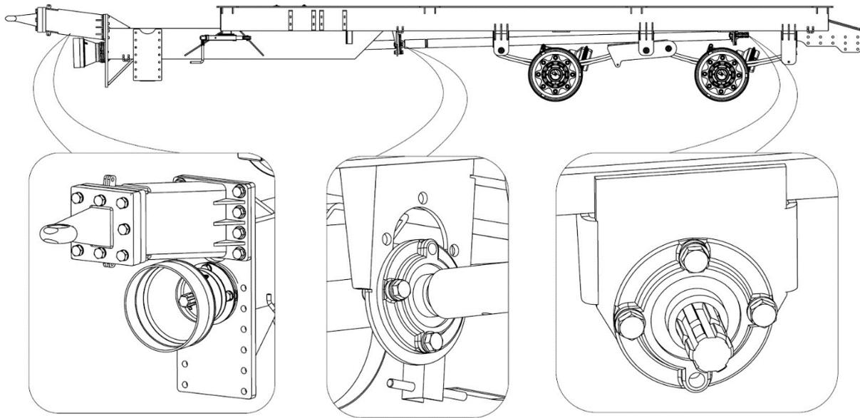
**Figure 17.** Position suitable for connection to the tractor's lower hitch
