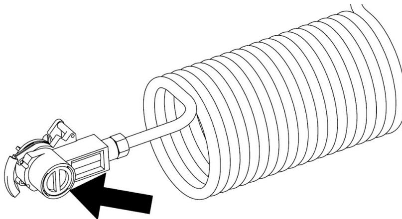
**Figure 39.** Knorr-Bremse brake system air filters
